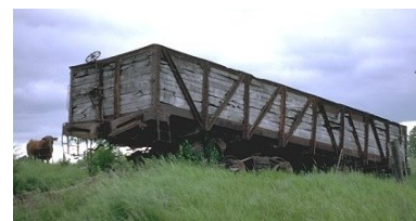
Composite gondola at Ash Grove Cement in Chanute, KS Photo by Evan Werkema
